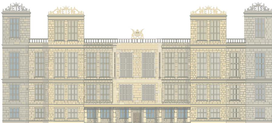
Front elevation illustrating the slightly taller outer towers and emphasising an uncompromising symmetry in contrast to the asymmetrical plan of rooms
